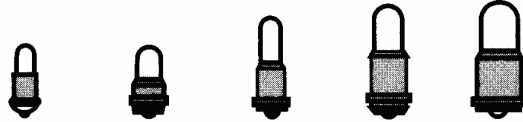
④① ④② ④③ ④④ ④⑤ T 3/4 T1US T1French T1 1/4 T1 3/4 2.5 x 9.5 3.17 x 9.5 3.7 x 14 4.5 x 16 6 x 16
