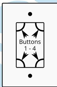
2x4 | 95 x 145mm Covers standard 2x4 wall recess
